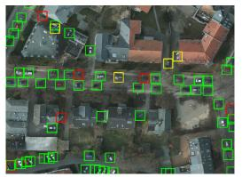
Areal imagery can be used to identify where cars are parked and when. Machine learning approaches can distinguish between cars and larger transport vehicles that, when combined with charging profiles and preexisting network topology, give qualified estimates of future loading scenarios.
